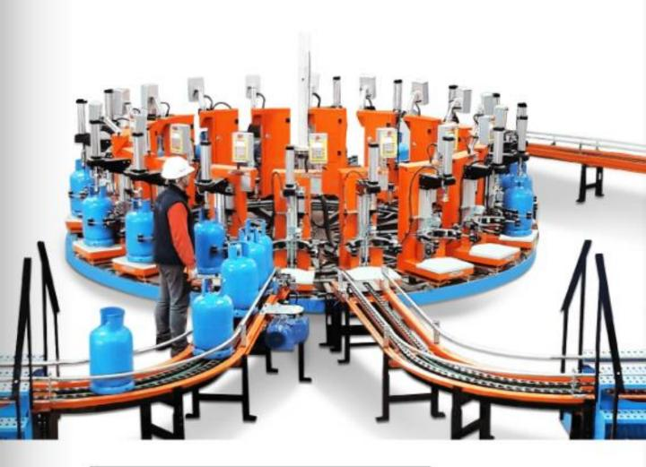
DM electronic filling carousel is used for big capacity lpg cylinders' filling.
